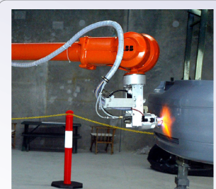
Flame Treatment Of A Bumper Fascia
